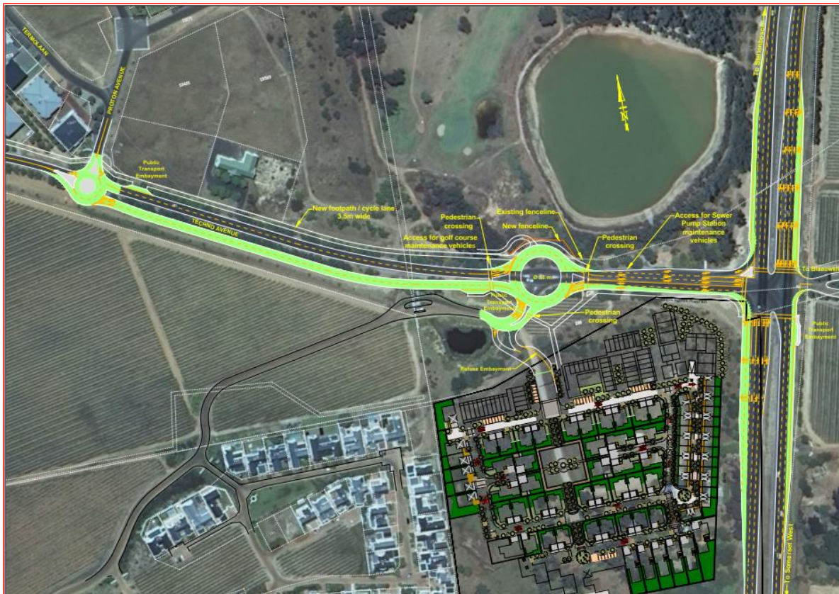
Figure 6-14: R44/Techno Avenue approved upgrades
